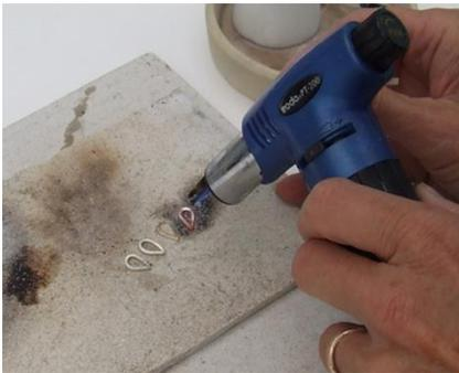
Solder each drop at the angle where the wires meet. Do several at a time and make sure that they have plenty of flux on them. Use a fine flame and hard silver solder as there is another solder joint to make later. Put each drop in the pickle to remove flux, wash and dry thoroughly.
