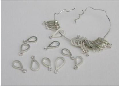
Pickle, wash and dry drops. Clean the flat surfaces with a buff stick if you think any need tidying up. Thread all the drops on a piece of wire and polish in a barrel polisher. If you want you can polish them on a polishing wheel although it is fiddly and time consuming. I have not given my drops a high shine finish.
