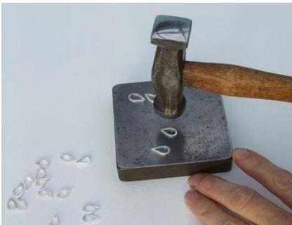
File off any excess solder and then hammer flat on a flat plate with a planishing hammer. Make sure the hammer has a polished surface so that the silver is not marked. The drops need to be as flat as possible to make sure that the resin will not seep under.
