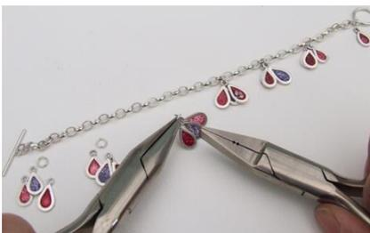
Solder toggle catch to chain bracelet. Group the tear drops in threes and attach each group with a jump ring made from 0.8mm round wire. Attach evenly along the bracelet and attach one drop next to the catch ring. The jump rings cannot be soldered on because the resin would burn with the heat of a torch.
