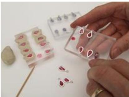
When the resin is hard, clean away the Plasticine and gently lift the drops by levering up the jump ring. The resin will not stick to the acrylic block. If the resin has seeped under the silver it can be scraped off with a finger nail- do not use anything sharp which will scratch the silver. If desired the silver and resin can be polished with micro-mesh polishing cloths.
