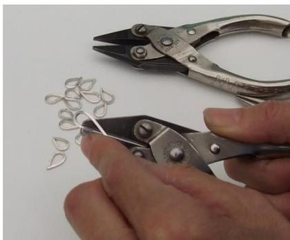
Use round pointed and parallel pliers to turn up 19 little tear drops from the square wire. They do not need to be the same shape but should be roughly 10mm long on the outside. Make sure the sides are straight by squeezing with the parallel pliers. The two sides should overlap one on top of the other.
