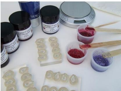
Make 3 pots of sparkle resin - lilac, pink and red. Use 1.4gm of each resin to 0.7gm hardener. Resin should be mixed 2 parts to 1 part hardener by weight for resin to cure (or set) properly. Follow safety instructions and wear a suitable barrier cream to protect your hands and work in a well-ventilated room.
