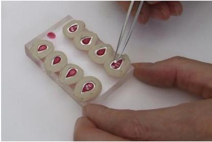
After an hour check test the sample dot to see if the resin has gone tacky. When it is tacky add some cubic zirconias to one of the red sparkle drops with tweezers. If you add the cubic zirconias before the resin is tacky they will sink and fall over - then they will not sparkle. Leave the resin to cure hard overnight in a warm dust free place.
