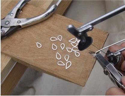
Cut the excess off by cutting along the side of one of the sides. This means the wire will be cut at the correct angle to meet the other side. Twist the wires with pliers so that they meet and adjust if necessary so that there is no gap between them. By doing this you do not have to file an angle.
