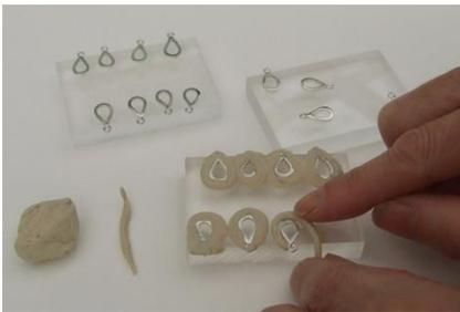
Divide the drops into 3 and attach them to acrylic blocks with Plasticine round the edges. Position them so that the jump rings stick out over the edge slightly. It is important to have the drops as flat as possible with no excess Plasticine under or over the drops. Pick up the acrylic blocks and look from underneath to make sure there are no gaps where resin could seep through.
